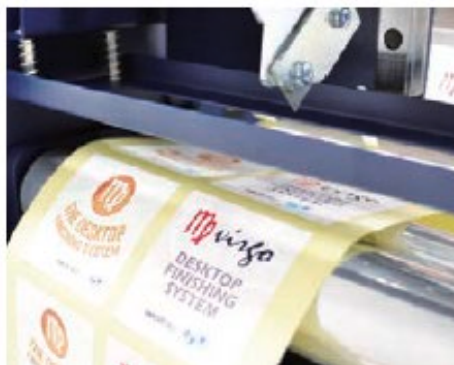
Pull the media through the aluminium rollers.
