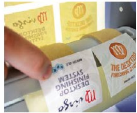
Attach the labels to the core using a waste label.
